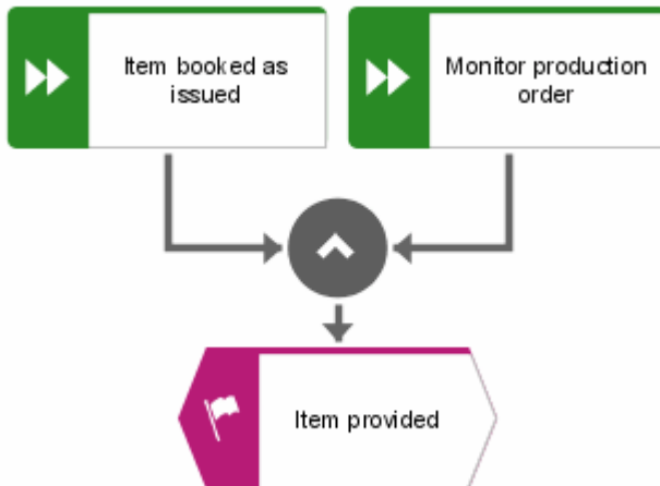
Figure 78: AND operator of functions with created events
