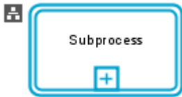
図 165: Symbol for a collapsed transaction
