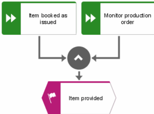
Figure 78: AND operator of functions with created events
