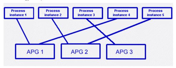
In this scenario, one node can become overloaded, for example, if nodes stop running and the other nodes have to take over.
