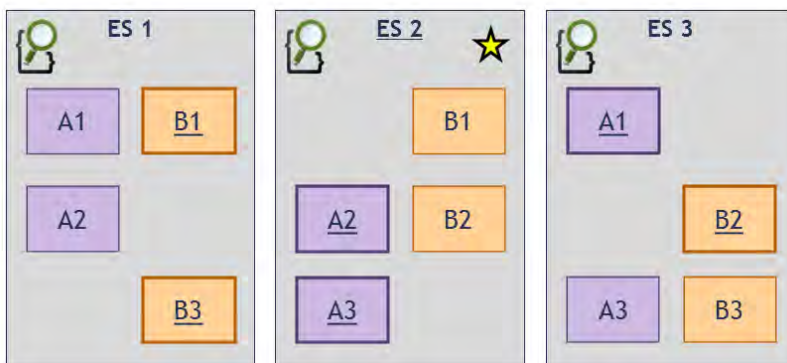
Figure 31: Distribution of primary and replica shards in an Elasticsearch cluster
