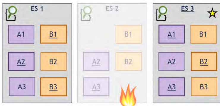
Figure 33: Handling of a failed instance
