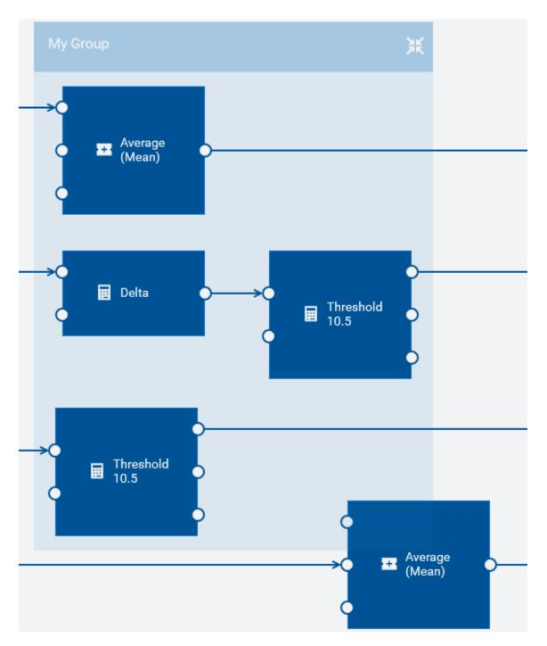
The size of the box that is shown for a group is determined by its contents. If you move a block within the group to a different position, the box size is automatically adapted (that is, the box is made larger or smaller). The same applies if you change the path that a wire takes to another block within the same group.
