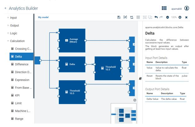
The palette on the left contains the blocks that you can add to your model. It has several expandable/collapsible categories for the different types of blocks.
