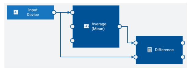
When the device measurement is received, the **Average (Mean)** block calculation is completed to generate an average before the **Difference** block computes the difference between the value and its average.
