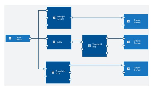
An input block which shows **Input Device** as the device name
