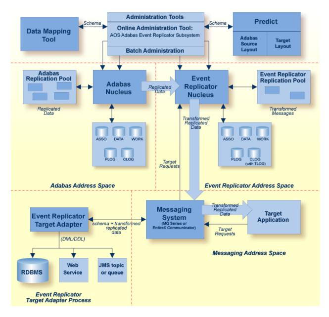
Once appropriate Event Replicator subscription and destination definitions are activated and the Event Replicator Target Adapter is started, normal processing for the Event Replicator Target Adapter will transform and apply replicated data to a relational database as the data is processed by the subscription. In addition, you can manually submit requests to the Event Replicator Target Adapter that:
