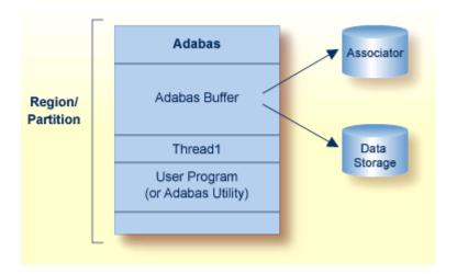
Multiuser mode is in effect when the Adabas nucleus is located in a separate region. It is the most efficient and therefore the recommended mode of operation.
