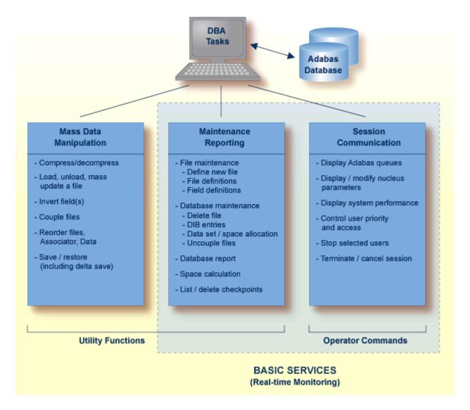
Basic Services makes it possible for the DBA to interactively monitor and change aspects of an Adabas database while an Adabas session is active. Using menu options or direct commands, the DBA can view resource status and user queues, display and revise space allocation, change file and database parameters, define a new file online, and stop a selected user or current Adabas session.
