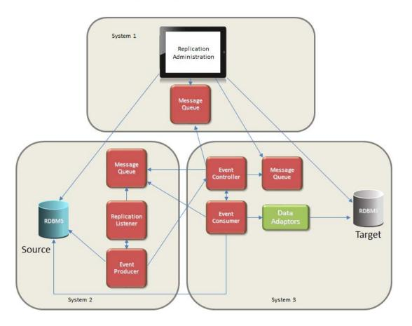
In the diagram, the replication components are spread across three different servers. In larger environments where there is a heavy transaction load or the source database is consuming all of its server's resources, it is recommended that the replication components be installed on a separate server.
