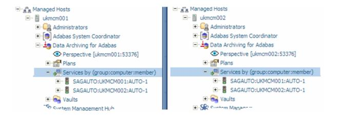
In the picture (above) we can see snippets of separate SMH sessions with ukmcm001 and ukmcm002 (our example computers). Now that the manual group definitions reciprocate, and the firewall obstacle is removed the daemons running in each computer are visible in every collaborating computer.
