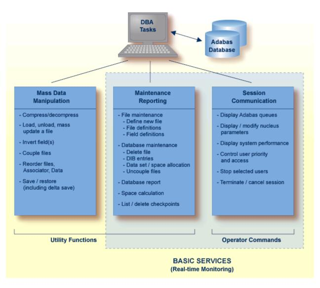
Basic Services makes it possible for the DBA to interactively monitor and change aspects of an Adabas database while an Adabas session is active. Using menu options or direct commands, the DBA can view resource status and user queues, display and revise space allocation, change file and database parameters, define a new file online, and stop a selected user or current Adabas session.
