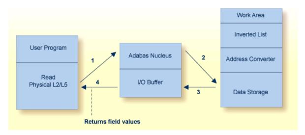
*ISN* sequence retrieves records in ISN order. Adabas uses database query commands (S*x*) to build and sort ISN lists, which can then be read using L1/L4 commands with the GET NEXT option. When reading, Adabas uses the address converter to find the RABNs of each ISN in the list and then reads and returns the records from Data Storage.
