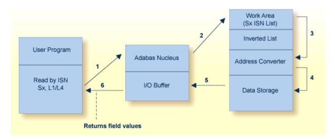
*Logical* sequence retrieves records by descriptor value. Adabas finds the value(s) in the inverted list, uses the address converter to find the RABNs of the ISNs related to the value, and retrieves the records from Data Storage.
