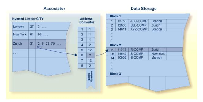
When a record moves or is deleted, Adabas updates the address converter automatically and transparently.
