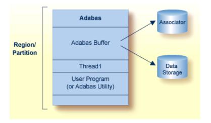
Multiuser mode is in effect when the Adabas nucleus is located in a separate partition/region. It is the most efficient and therefore the recommended mode of operation.
