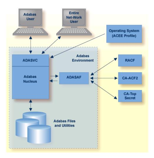
The central security logon ID is used to log on to the system. Through the operating system or TP monitor, the installed external security package package performs authentication of the logon ID. For calls from a remote workstation or non-IBM platform, a remote logon procedure is used to give the logon ID to ADASAF.
