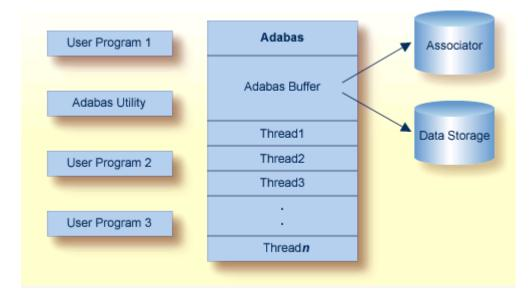
When using Adabas in multiuser mode, interregion communication is handled by Adabas in a manner that takes optimum advantage of the communications facilities offered by the various operating systems.
