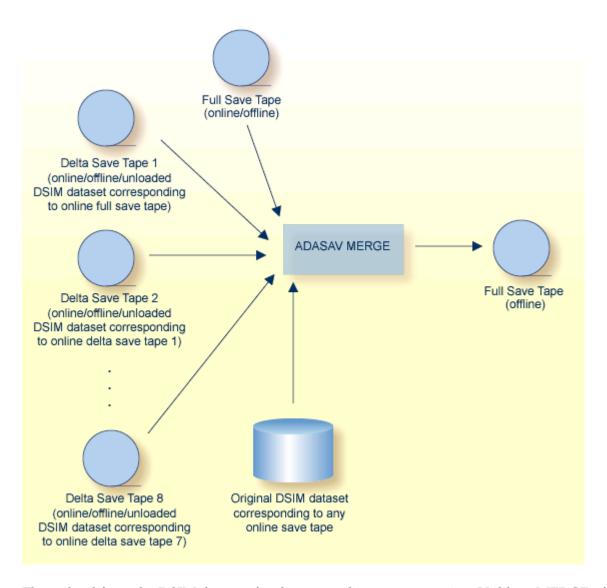
The unload frees the DSIM data set for the next online save operation. Unlike a MERGE of the DSIM data set, its "unload" eliminates the need to process the associated online save data set-which may be very large in the case of a full save-again just after it has been created.
