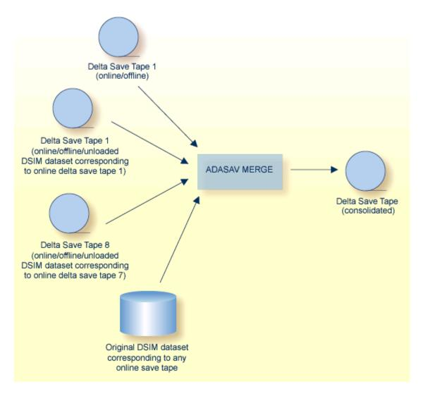
The original DSIM data set corresponds to any online save input. Any online delta save input to which the original DSIM, if supplied, does not correspond must be followed (with the next higher sequence number) by the corresponding unloaded DSIM.
