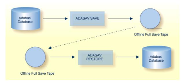
The graphic shows the general sequence of a conventional Adabas database offline save operation without Delta Save. First, the ADASAV utility's SAVE function is used to create a full database save (SAVE database), usually on tape. If the need arises, this full database save can be used for restoring either the entire database or specific files to their state at the time of the save operation (using the ADASAV RESTORE function).
