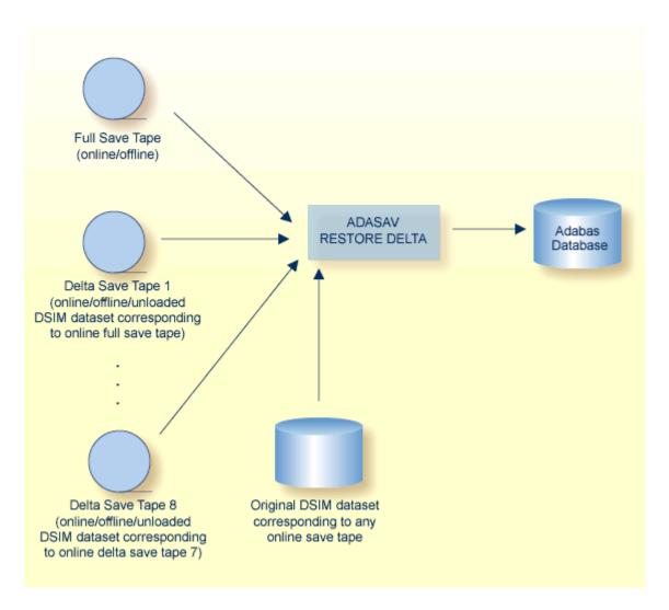
Consecutive saves must be specified for RESTORE DELTA: no save tape may be missing. Each save tape may itself be the output of an earlier merge operation. For tapes that originate from online save operations, the corresponding original or unloaded DSIM data set must be specified. An original DSIM data set is *not* reset at the end of the RESTORE DELTA operation but remains available for further merge operations.
