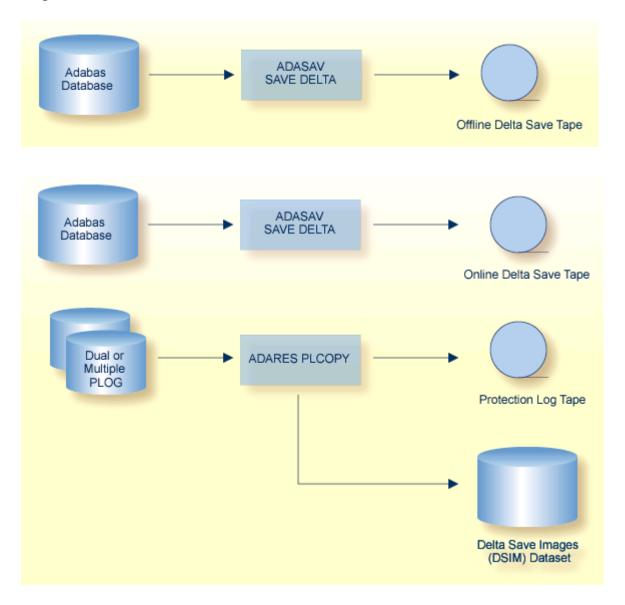
Online Delta Save Tape shows that the online delta save-like a full save-results in protection log (PLOG) output for any activities performed while the delta save was in process.
