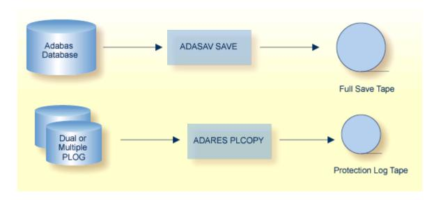
If required, the entire database or specific files can be restored to the state at the end of the online save operation by using the full database save tape together with the associated protection log as input to the ADASAV RESTONL function, as shown below.
