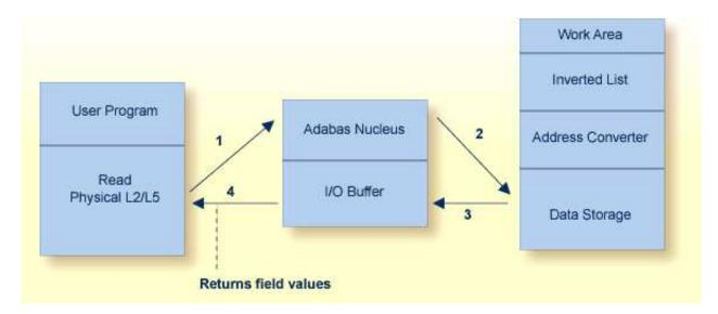
*ISN* sequence retrieves records in ISN order. Adabas uses database query commands (Sx) to build and sort ISN lists, which can then be read using L1/L4 commands with the GET NEXT option. When reading, Adabas uses the address converter to find the RABNs of each ISN in the list and then reads and returns the records from Data Storage.
