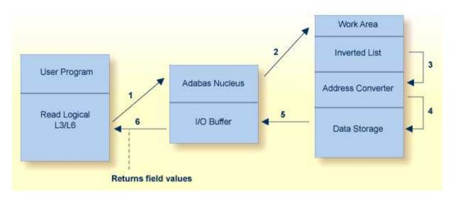
Reading in logical sequence retrieves all the records related to a single value or a range of values of the specified descriptor. It returns the records sorted in ascending/descending order by descriptor value, and in ascending/descending ISN order within each value. You can specify a starting and ending value. You can also specify the field(s) for which values are returned. Read logical is useful when you want the returned records sorted on a particular field.
