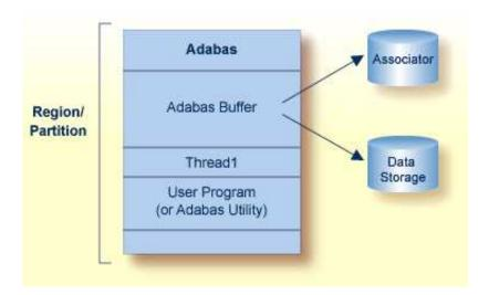
Multiuser mode is in effect when the Adabas nucleus is located in a separate partition/region. It is the most efficient and therefore the recommended mode of operation.
