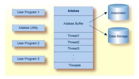
When using Adabas in multiuser mode, interregion communication is handled by Adabas in a manner that takes optimum advantage of the communications facilities offered by the various operating systems.
