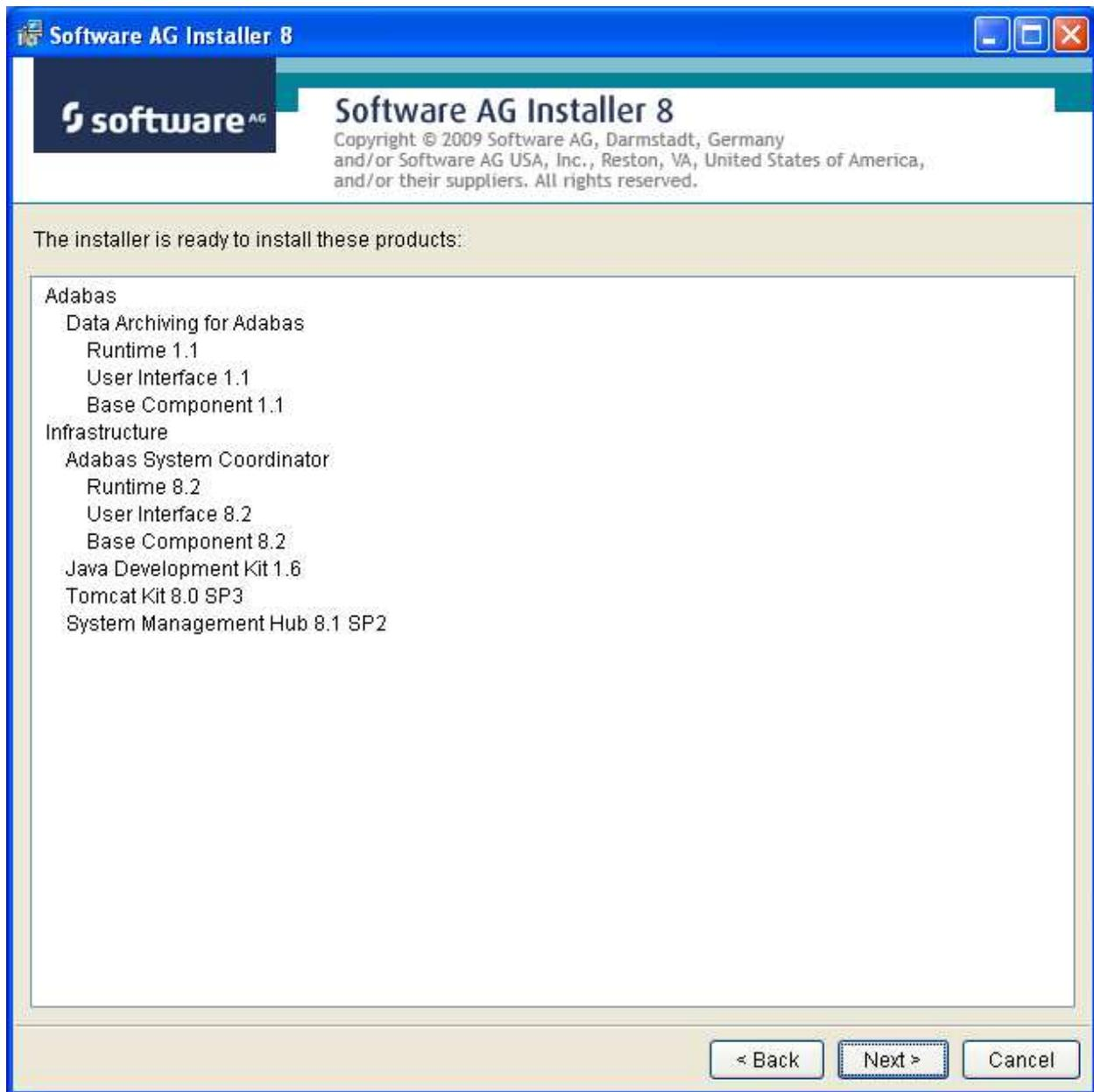
The installation may take some time. In the case of Data Archiving for Adabas the installation is usually quite quick whereas the install of the prerequisite System Management Hub (for installing the User Interface) takes longer.
