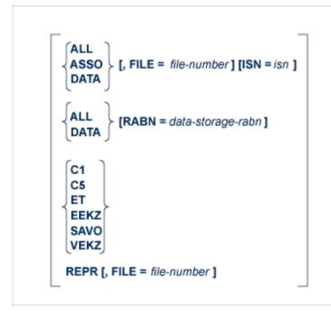
The IPLOGPRI function is used to print the sequential intermediate data sets created from the PLOG merge process. Input to ADAPLP IPLOGPRI must be a MERGINT1/MERGINT2 data set created by the ADARES utility and is specified in the DDPLOG DD JCL statement. Operation is similar to the SPLOGPRI function.
