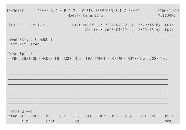
2 Make any necessary modifications and press PF5 to confirm (modify only).
