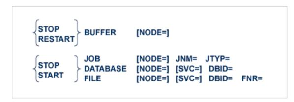
Once the STOP BUFFER command is accepted, the buffer manager initiates the stop process, and it is then no longer possible for batch services to start the buffer.
