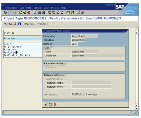
The Appl\_Object element points to the business object instance to be created in SAP. In this case, the event parameter IDOCORDERS.inputFinished.Appl\_Object corresponds with business object SalesOrder (BUS2032). Therefore, events IDOCORDERS.inputFinished and BUS2032.created can be correlated easily because event IDOCORDERS.inputFinished already comes with a reference to business object type BUS2032. The same applies for events IDOCORDCHG.inputFinished and BUS2032.changed.
