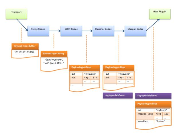
Apama provides a selection of codecs by default for converting from common formats and for use with customer-provided codecs to provide standard transformations. The above diagram uses the following standard codecs:
