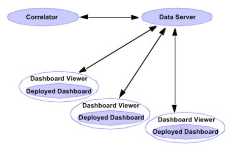
With the Dashboard Viewer, dashboards communicate with the Dashboard Data Server, which communicates with the correlator.
