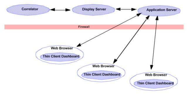
Locally-deployed dashboards communicate directly with the data server.
