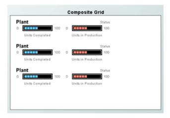
Unless you have created or deleted instances of the tutorial DataView, there will be three instances of the Composite object in the grid. They do not show any data because the sample rtv file is not attached to the data of the tutorial DataView.
