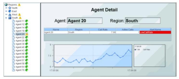
You can optionally configure tree control icons, using images of your choice, to visually indicate the type of elements in the tree, for example, Production or Sales, whether the element is in a critical state, and to also propagate the status of priority elements to the top of the tree. See "Configuring tree control icons" on page 166.
