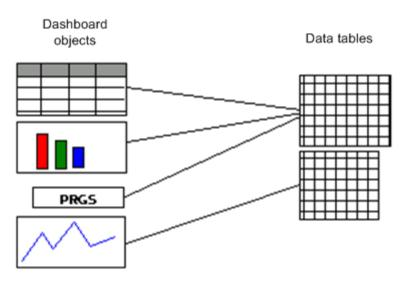
When a DataView field changes, the correlator generates an update event with details of the change. When this event is received by a dashboard, the dashboard updates one or more data tables and the changes are reflected in all attached objects.
