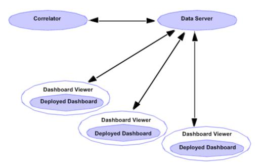
You can scale your application by adding data servers to your configuration. Each correlator can communicate with multiple data servers, and each data server can communicate with multiple correlators.
