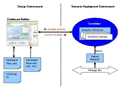
In order to use Dashboard Builder to create a dashboard for a DataView, you need to start a correlator and inject the DataView into it. You should use a development correlator to initially develop dashboards, not a deployed correlator acting on live data.
