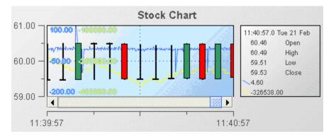
Overlays can be hidden by tuning off the overlayNVisFlag property. This is for use when building dashboards where you will have input controls such as checkboxes which will allow the user to hide or show different overlays.
