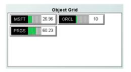
Here the grid is using one of the label object types in order to display the **Instrument** and **Price** variables of the tutorial DataView instances. The label object used provides a graphical indication of the price as well. There is one instance of the label object for DataView field. If a new instance is created, an entry for it would automatically be added to the object grid.
