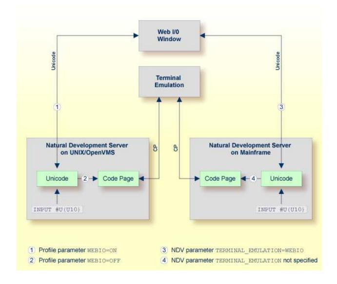
So that the Natural Web I/O Interface client can be invoked, the Natural Development Server has to be configured as follows:
