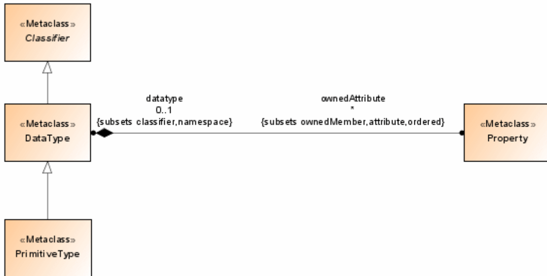
Figure 40: DataTypes diagram from the UML specification
