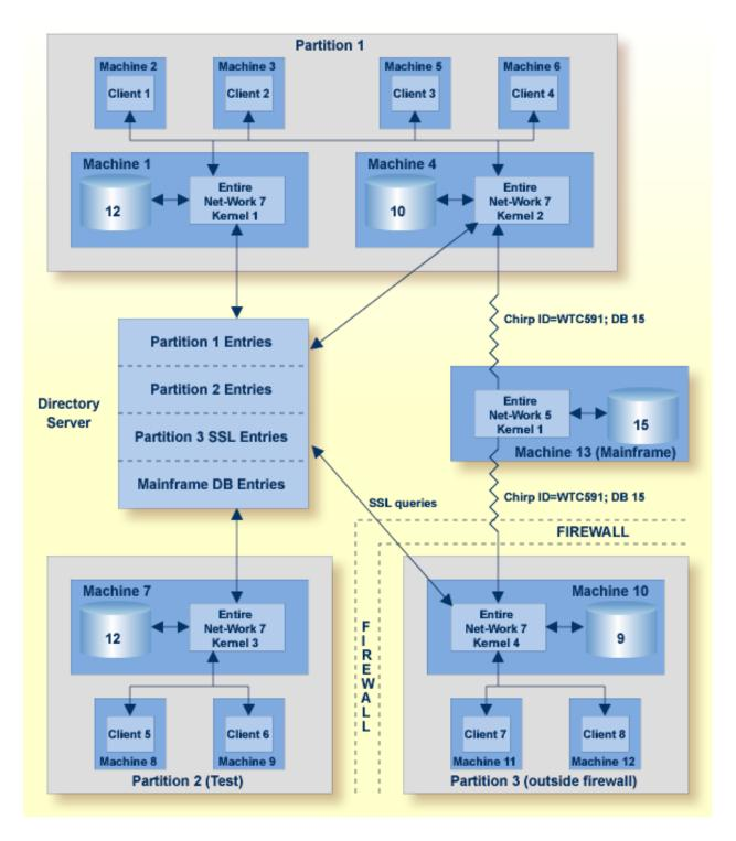
In this diagram, partitioning is used to:
