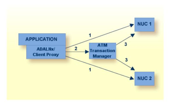
1. The application communicates with its target Adabas databases in the normal way. The client proxy monitors the commands issued by the application, selecting any that are transactional and reacting appropriately.
